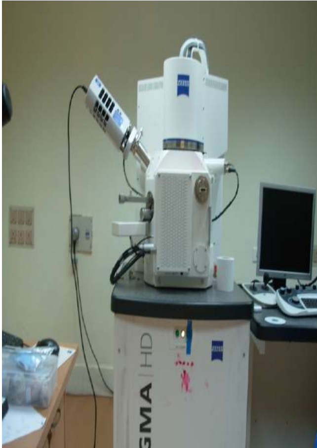
FESEM with EDS & Straining stage
