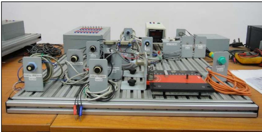
Test setup for inductive and capacitive type proximity sensors
