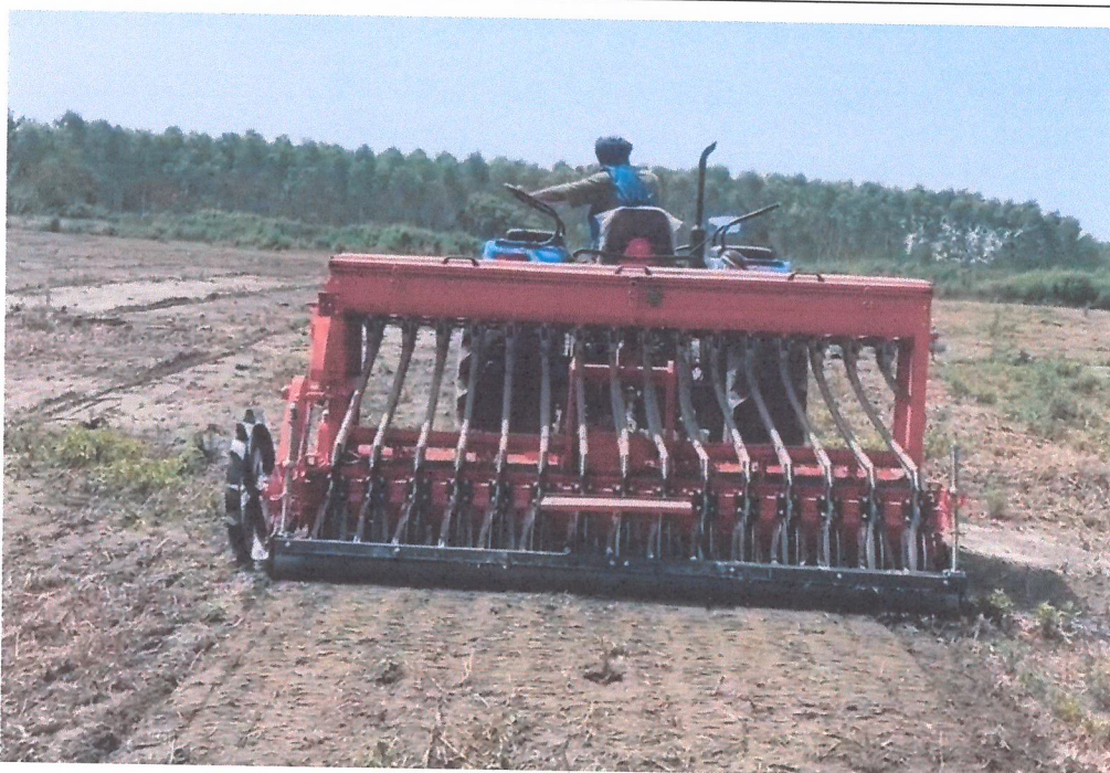
Fig.17 Testing of tractor operated super seeder
