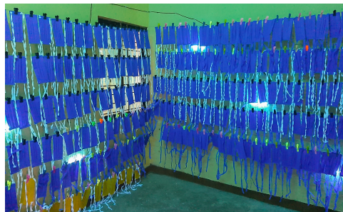
Figure 6: Developed facemasks being sterilized by UV-C light at CSIR-CMERI.
