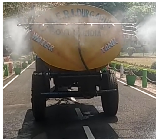
Tractor operated road disinfection spray system
