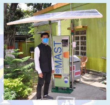
triggers audio-visual alarm and enters into the third phase. The system then prompts for I-Card of the person and if machine detects a valid I-Card, it dispenses one set of facemask to the person and sends his / her details by e-mail to the pre-defined authority for necessary action. The IntelliMAST is designed to be deployed in the outdoor environment and powered with integrated solar setup and electrical grid for 24x7 operation.
