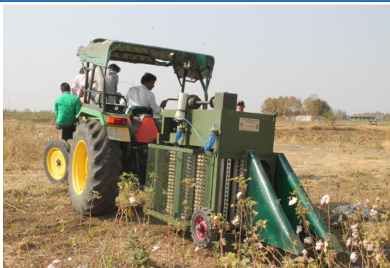
Fig.2. Spindle type picking head fabricated at CoEFM, Ludhiana
