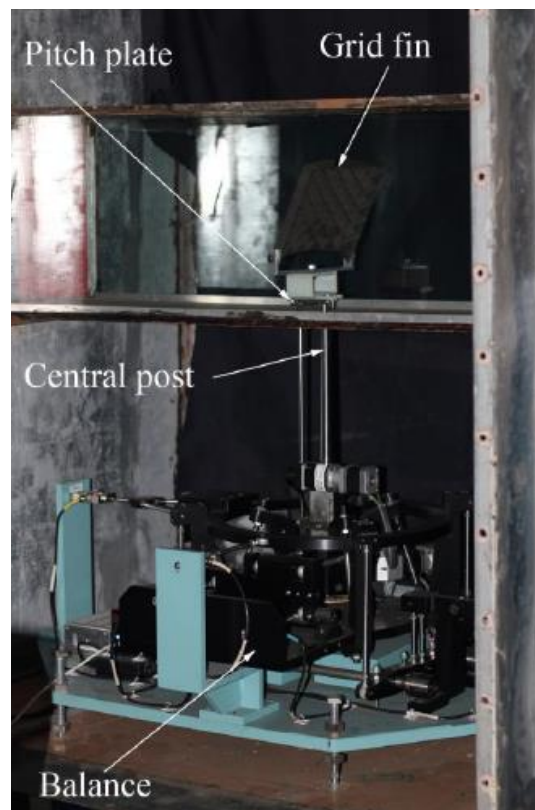
Measurement of aerodynamic forces and moments of grid fins
