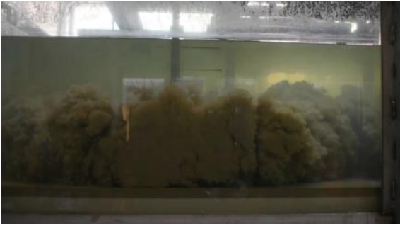
Observation of off-bottom suspension of gypsum particles
