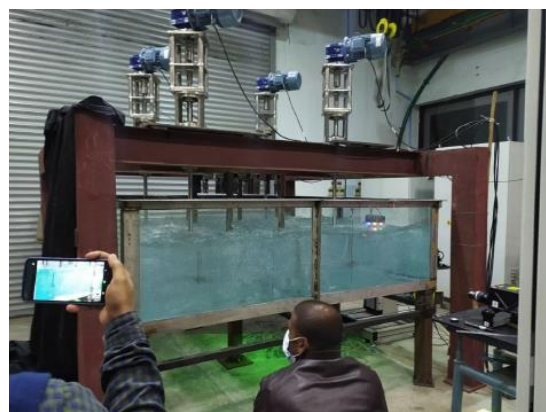
Measurement of vertical velocity close to the wall using PIV
