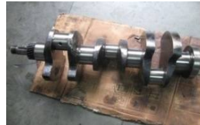
Photo of ADI Crankshaft after 500 hrs test
