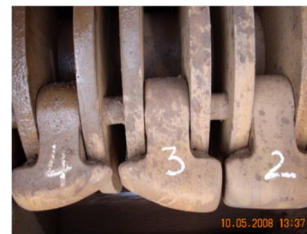
Crusher fitted with ADI hammers After 158 hrs of operation
