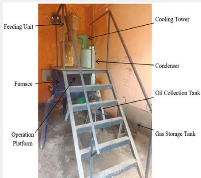
Figure 9: Polymer Waste Pyrolysis Unit at CSIR-CMERI (Capacity: 20kg/batch)
