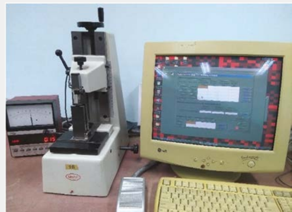
Figure 1: Setup of calibration for block gauge comparator (Reference EAL-G21)
