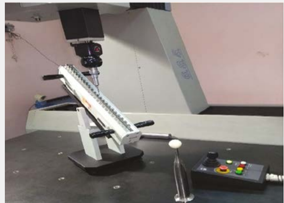
Figure 2: CMM being calibrated by Step Gauge
