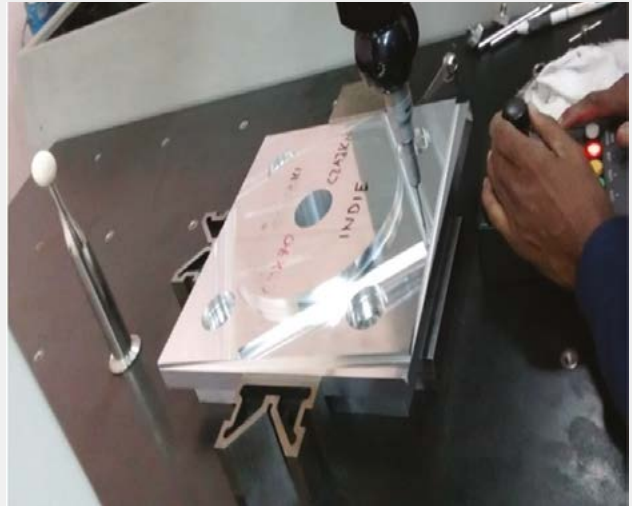
Figure 3: Test sample of Universal CNC Milling Machine being measured by CMM
