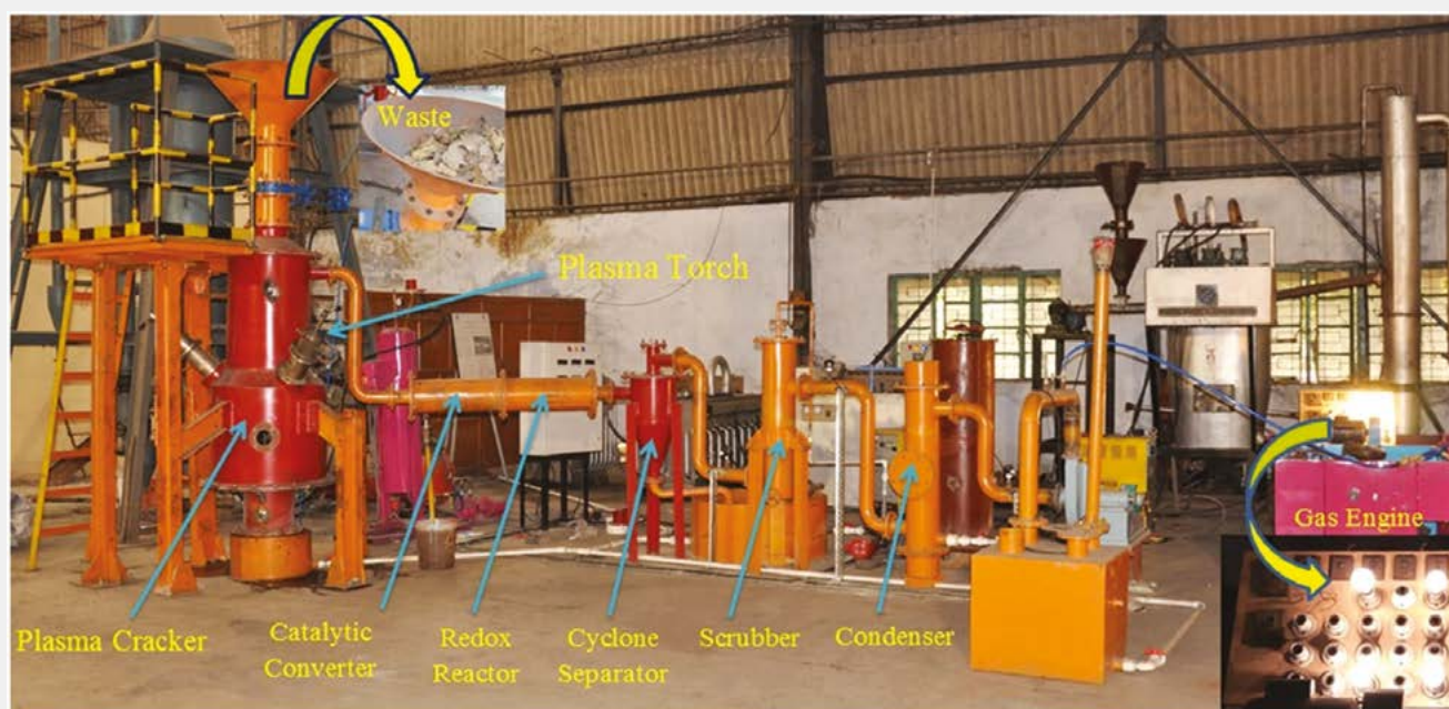
Figure 7: Plastic Disposal Unit at CSIR-CMERI (Capacity: 25 kg/hr)
