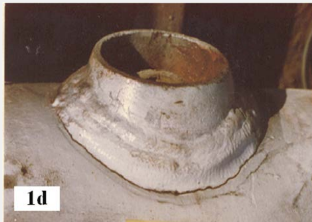
Figure 1d: Crack on Boiler Superheater
