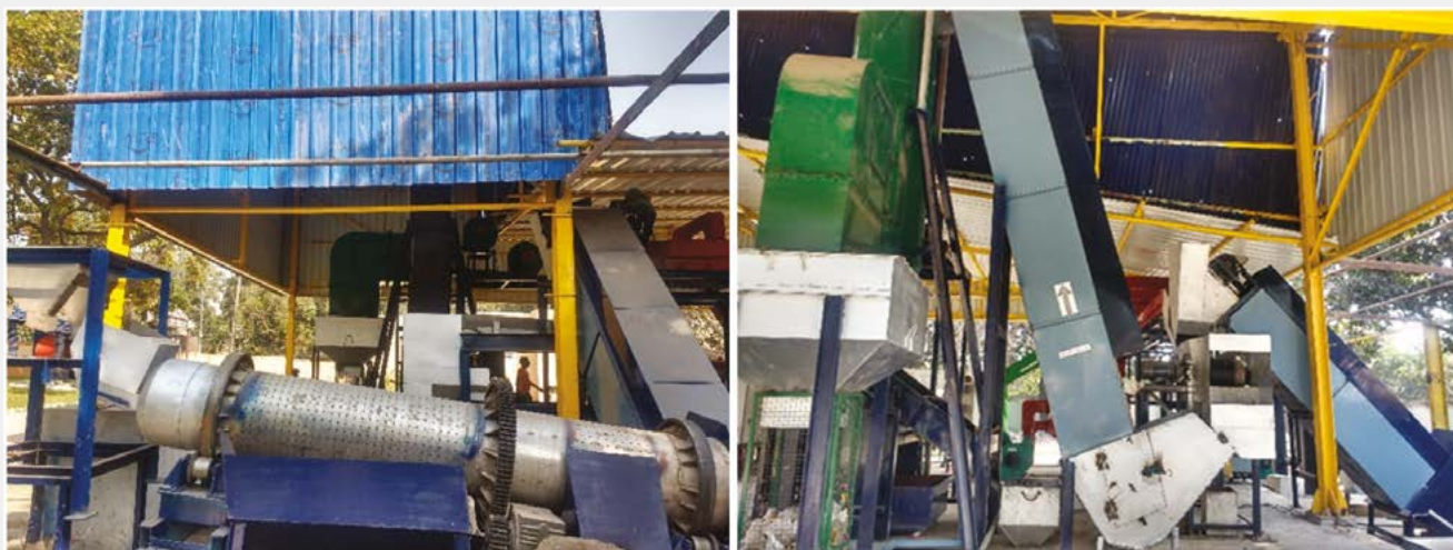
Figure 5: Mechanized Segregation Unit for Dead Waste at CSIR-CMERI (Capacity: 100 kg/h)
