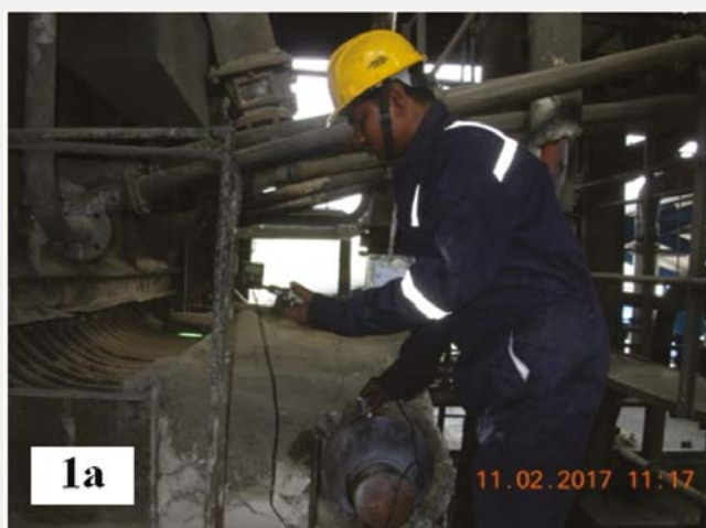
Figure 1a & 1b: Non-Destructive Examination of the critical components on site
