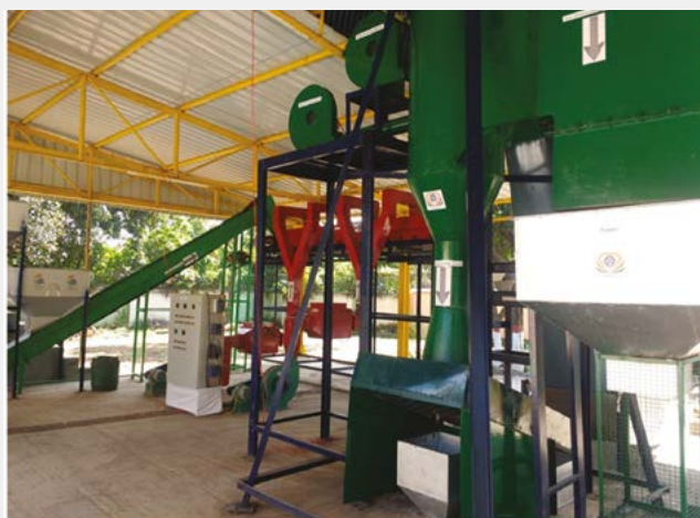
Figure 3: Mechanized Segregation Unit for Live Waste at CSIR-CMERI (Capacity: 50 kg/h)
