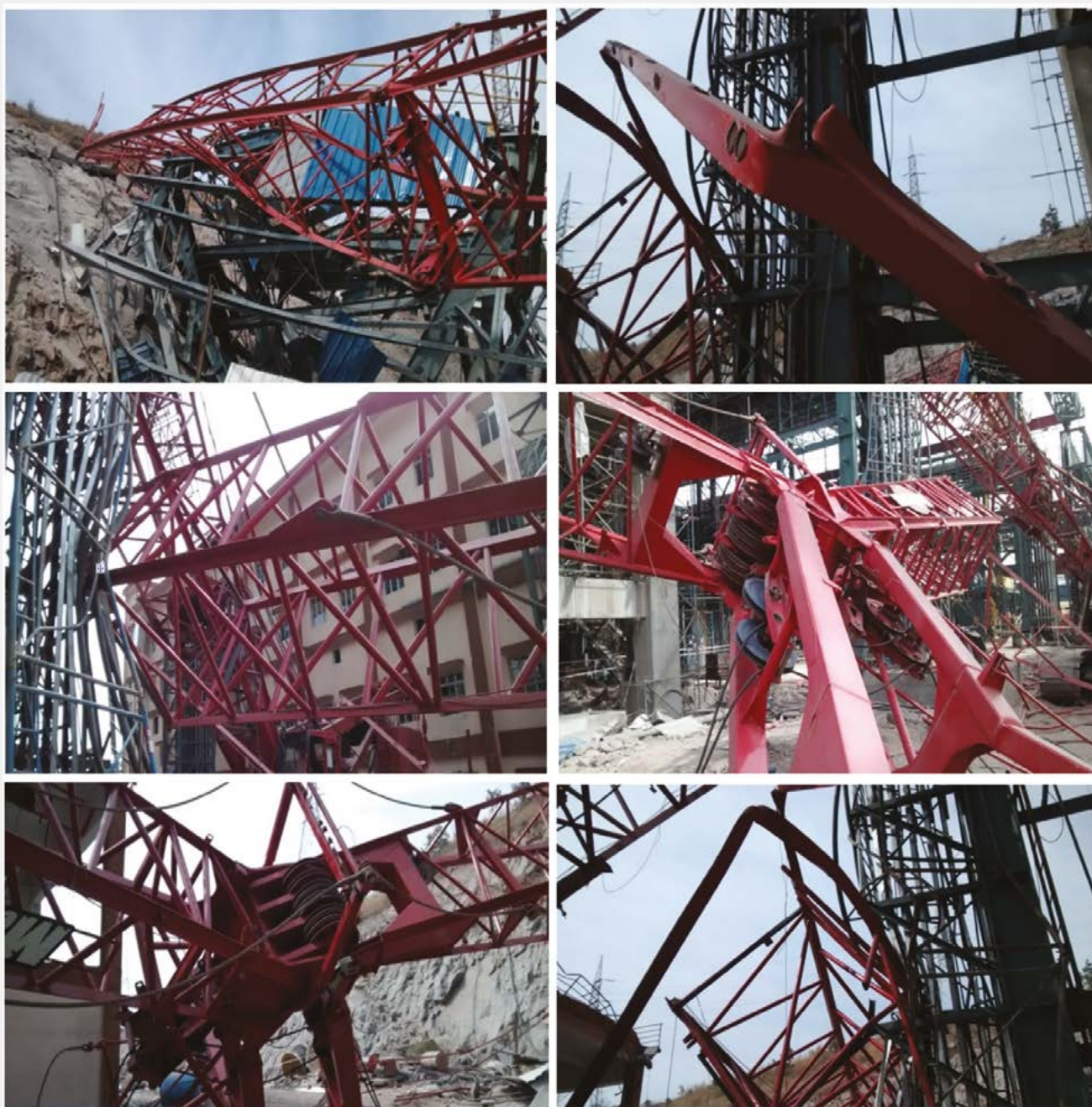
Figure 3: Catastrophic failure of the crane boom of 225 ton crane at Hindustan Zinc Limited, Udaipur, Rajasthan Site
