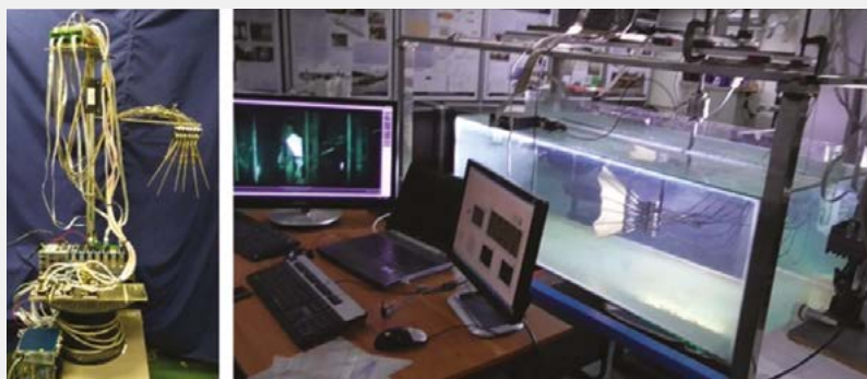
Figure 4: (Left) Multi-ray caudal fin prototype without web, (Right) execution of identified motion primitives in water by the developed caudal fin prototype
