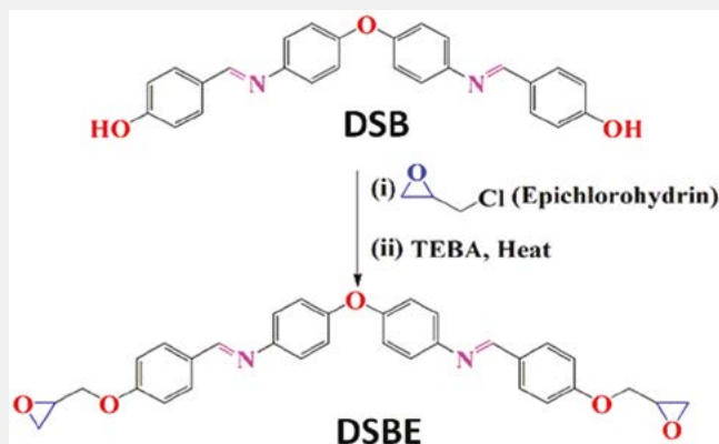
Figure 10: Synthesis of Schiff base epoxy (SBE) from Schiff base (SB)
