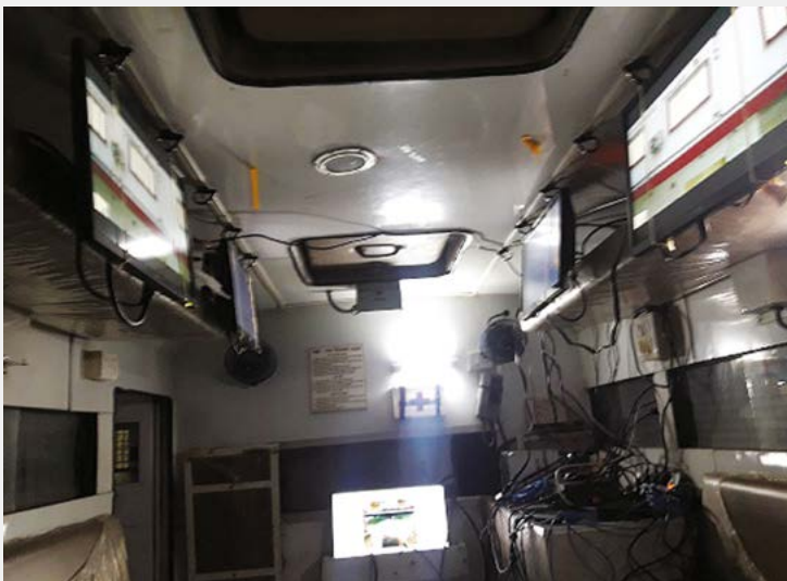
Integration and testing of electronics & communication systems inside MCV Prototype – Bus Type (Robotics and Automation Group)
